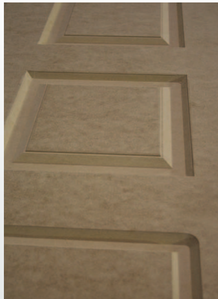
CNC ROUTERS ARE USED TO CREATE CURVILINEAR, ROUNDED AND 3-DIMENSIONAL PROFILES (AND CORNERS) OF SUBSTRATES IN PREPARATION FOR 3D LAMINATION.
